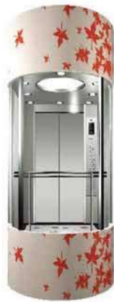
RJ100 (Standard) Car cover: Baked enamel steel plus color decoration patterns Observation Wall: Laminated Safety Glass Decoration Roof: Round acrylic lamp in the middle, downlights in the sides Car wall: Hairline Stainless Steel Handrail: Stainless steel tube Floor: PVC
