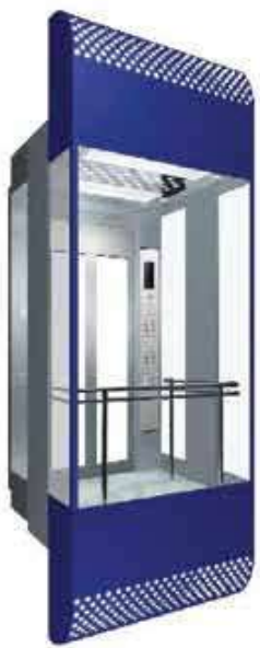
RJ102 (Optional) Car cover: Write acrylic decoration hood Observation wall: Laminated safety glass (three pieces) Decoration roof: Baked enamel steel frame and blue acrylic lighting strip Car wall: Hairline stainless steel Handrail: Stainless steel tube Floor: PVC
