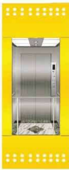
RJ101 (Standard) Car cover: Baked enamel with acrylic lighting decoration Observation wall: Laminated Safety Glass Decoration Roof: Hairline stainless steel frame, acrylic light-emitting panel, downlights Car wall: Hairline stainless steel Handrail: Stainless steel tube Floor: PVC
